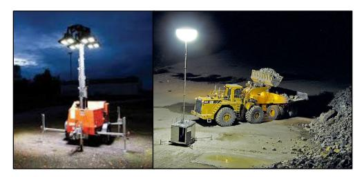
17.3.6 Quarry lighting is critical to health and safety and the security of quarrying operations particularly during Autumn and Winter months where hours of working will extend into dusk/darkness. It is possible to sub-divide the proposed extraction, processing and restoration works into 4 discrete areas to better understand the lighting requirements needed. These are as follows:
