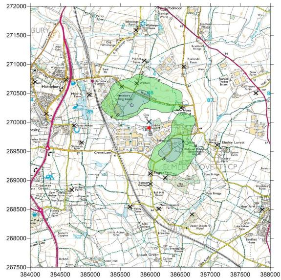
Figure 4: Short term Ground Level Concentration of  $NO_2$  (99.79th %ile of hourly means), Stack Emissions
