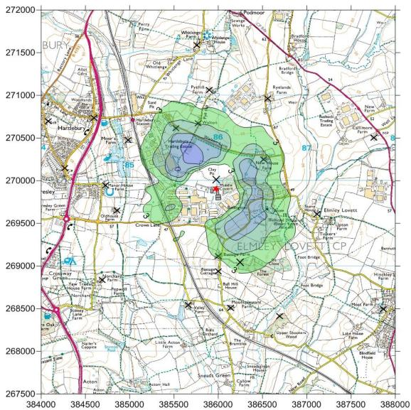
Figure 5: Short term Ground Level Concentration of  $SO_2$  (99.99th %ile of 15 min means)
