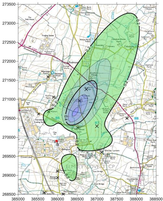
Figure 3: Annual Average Ground Level Concentration of  $\mathsf{NO}_2,$  Stack Emissions
